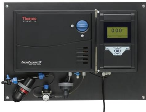
The Orion Chlorine XP analyzer measures free, total, and both free-total chlorine in water. Design features help minimize the need for periodic calibrations and offer compatibility with many disinfectant processes. It utilizes an optical DPD-reagent based measurement technology that can be configured to use the least amount of reagents while maintaining outstanding accuracy.
